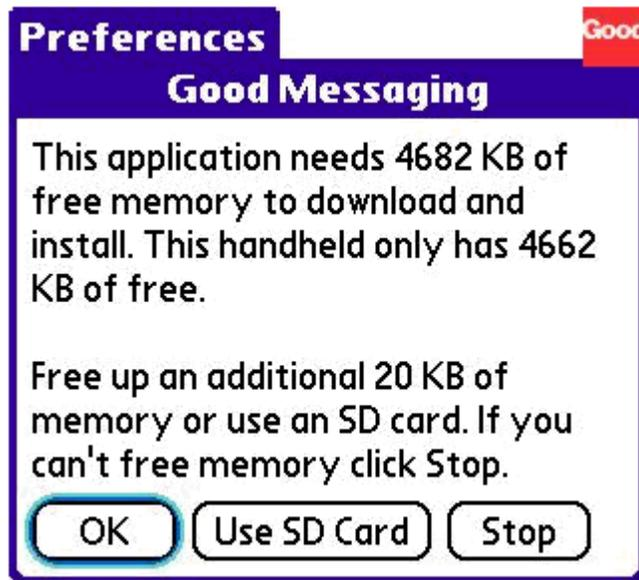
During an upgrade the Good Client checks to see if enough internal memory is present on the handheld to complete the upgrade. If the required memory isn't available, the user is prompted with this screen.
